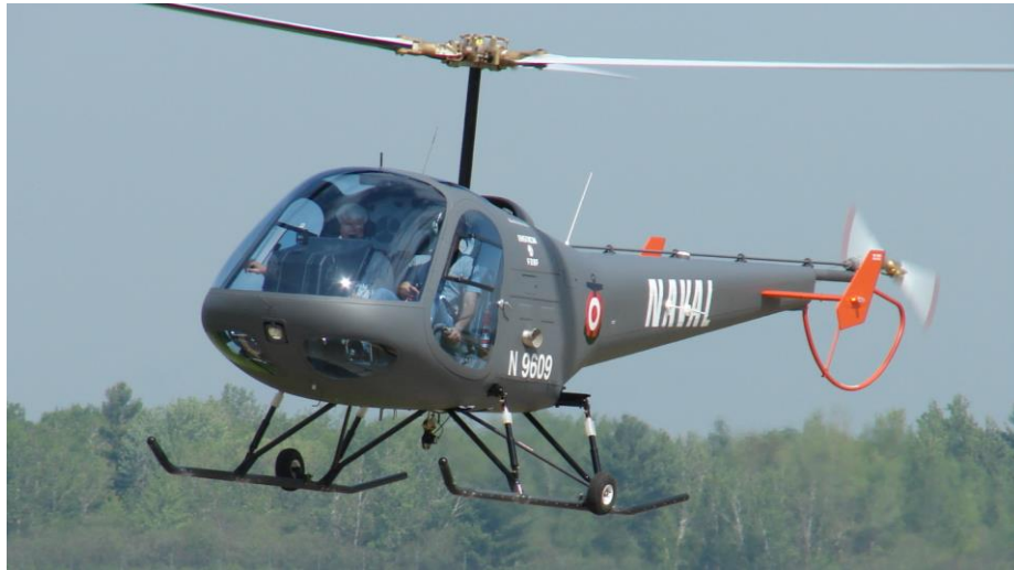
F28F – three-place, turbocharged, used for training, police patrol, general commercial work and personal/VIP transportation
