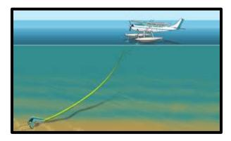
To set an anchor, it can be lowered down to the bottom paying attention how much line is used. Measurement marks can help. Then the amount of desired scope is played out and secured to a cleat. As the seaplane drifts downwind and the slack is taken up the fluke or blades dig in.
