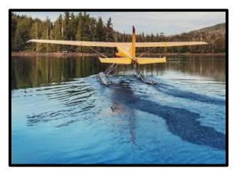
During turns the floats pivot at the location of the center of buoyancy (COB). At idle the float rides level in the displacement position with the COB located midway on the floats. At the COB we can identify the same point on the fuselage. The distance aft to the tail area is a long arm. So when at the level displacement position and winds are present the seaplane wants to weathervane into the wind much like a barn weathervane.
