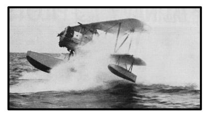
This can lead to catastrophic results with an upset, along with water, spray, and mist can be thrown in the propeller causing erosion and damage.
