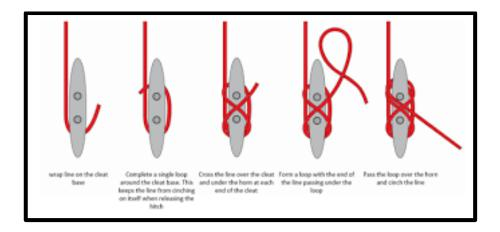
A cleat hitch can tighten as the seaplane tugs on it with wave motion. The hitch is easily loosened and removed when preparing to depart. If it becomes wet it is still easy to remove
